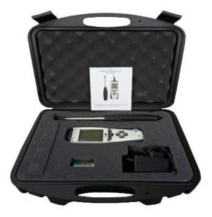
This hot wire thermo-anemometer is ideal for low air velocity and volume measurement. The slim plug in telescopic hot wire probe extends from 0.26 to 1.2m (inc handle) has a probe sensor head 8.5mm and is ideal for grille hoods and diffusers. It is excellent for ventilation surveys, air conditioning, clean rooms, flow hoods, air balancing and environmental monitoring.
