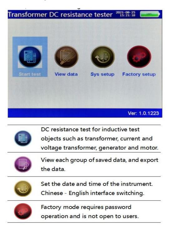
**GRDTek** 2. Choose "Start test", press "OK" to enter measurement interface, as below
