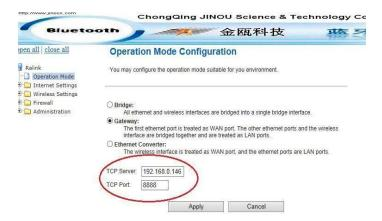
Enter TCP server IP address and TCP port number. Click "Apply" and wait for a few seconds until the page refreshes. Then re-power the gateway and the gateway will automatically connect to designated server.
